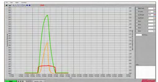
ProView PC software adjusts sensor parameters and log data.
